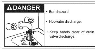
The water passing out of the drain valve may be extremely hot. To avoid being scalded, make sure all connections are tight and that the water flow is directed away from any person.
